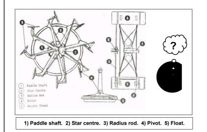
Paddle Steamer Waverley has two rimless paddle wheels, each with eight flat wooden floats, as were fitted to almost all the paddlers of the L.N.E,R. and its predecessor, the North British Railway.
